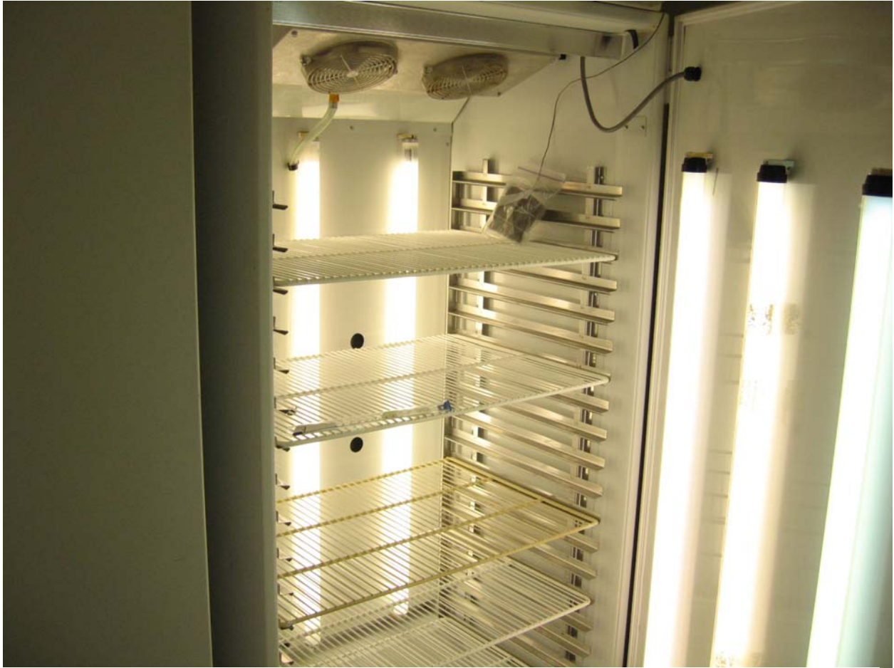
Image 3. Following the pre-chill treatment, the germination boxes were placed into a germination chamber maintained at 15/30° C darkness/light for 16/8 hour per day.
