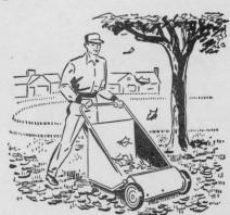
More and more folks are finding it worth while to invest in a lawn sweeper. The typical machine is an arrangement of revolving brushes mounted between two wheels. A wireframe canvas catcher is provided into which leaves and other debris are swept by the revolving brushes.
