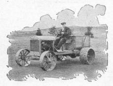
THE new Toro Junior Tractor equipped with a dump box, is a highly desirable tractor adapted to a wide range of work. The electrically welded steel body holds one full yard and makes it a convenient machine for all classes of hauling and general construction work on large areas of turf.
