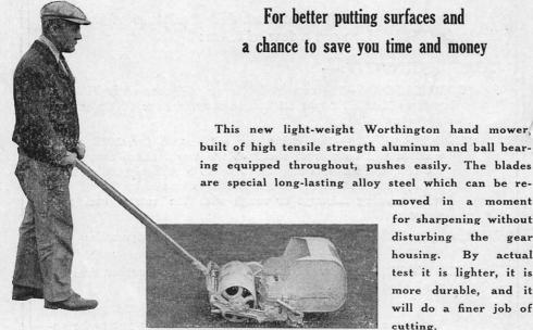
moved in a moment for sharpening without disturbing the housing. By actual test it is lighter, it is more durable, and it will do a finer job of cutting.
