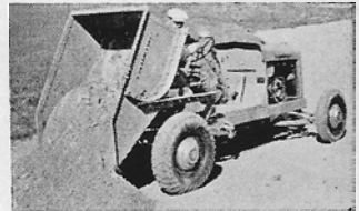
Rocker Type dumping load in sand trap. The body tilts back and returns to loading position automatically.
