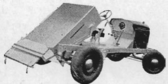
For those who prefer a rectangular type dump body with automatically opening and closing tail-gate, the model illustrated here is recommended.
