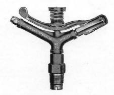
Rain Bird Sprinklers are of the slow rotating type driven by an oscillator forced outward by the stream and returned by a torsional spring causing an impact against the main nozzle that is positive and steady. There is never any whipping or uncertain turning. No internal mechanism to interrupt flow. This insures maximum coverage. Working parts are on the outside, always accessible and foolproof.
