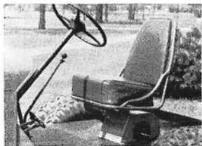
Here's a real comfortable fully upholstered bus seat mounted on a coil spring for easy riding.
