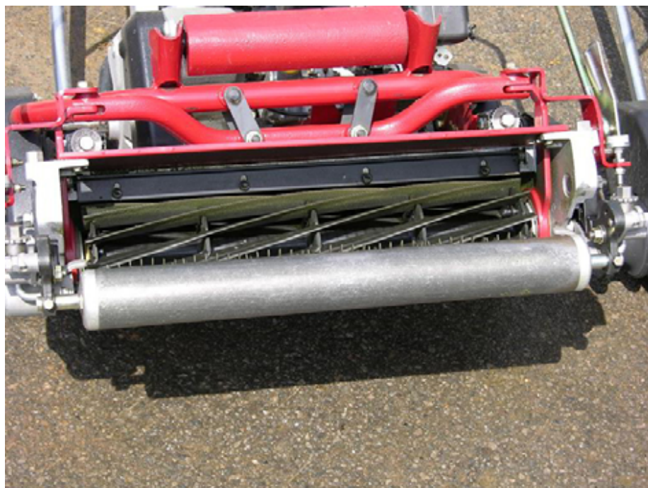
Many superintendents use solid front rollers on putting green mowers year-round to reduce mechanical stress to turf while providing excellent playing surfaces.
