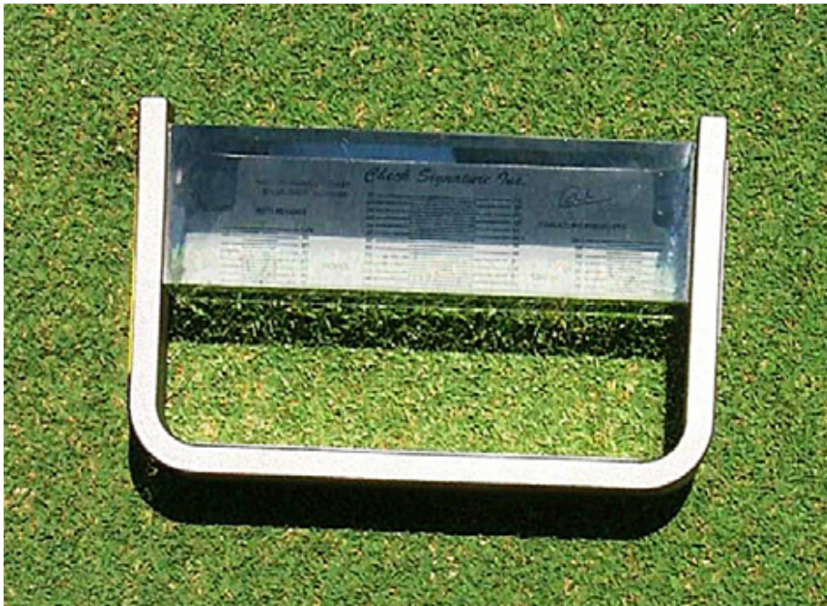
Know the actual mowing height in the field, and this can be accurately determined using a prism gauge. A mower's bench setting is just a starting point when adjustments in the field are needed in response to environmental conditions.
