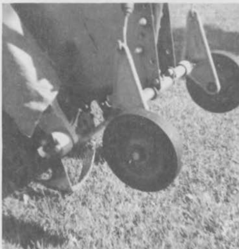
A sod knife blade cut in half. Used to cut shallow furrow to place telephone wires underground.
