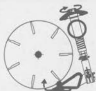
SINGLE KNOB, BEDKNIFE-TO-REEL ADJUSTMENT
