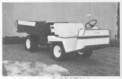
Powered by a 16 HP engine, the UV4 features a rugged torque converter transmission with 2 forward speeds, plus reverse, along with powerful hydraulic brakes. The box handles items 5 feet long and 4 feet wide. The tailgate hinges at the top and bottom for your choice of loading and dumping (dumping is done hydraulically with the flip of a lever).
