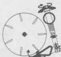
SINGLE KNOB, BEDKNIFE-TO-REEL ADJUSTMENT
