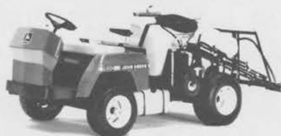
A single lever hydrostatically controls the 1800's direction and speed.
