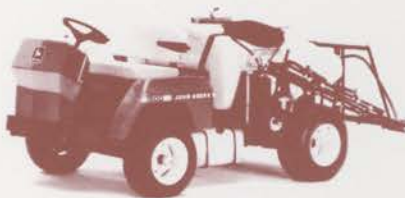
A single lever hydrostatically controls the 1800's direction and speed.
