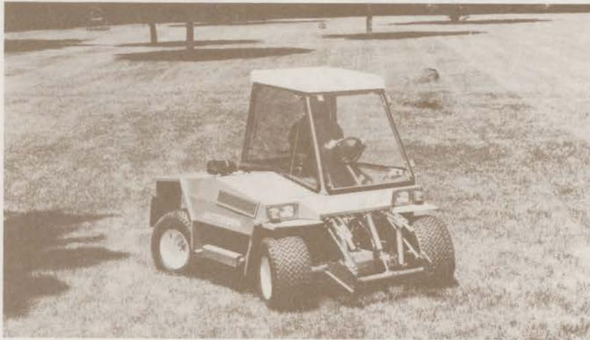
Four-wheel drive, four-wheel steering and a low center of gravity are key features of the new Jacobsen G-4 x 4
