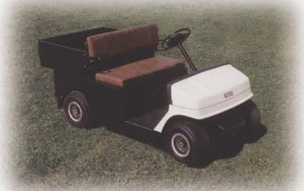
The G2: Yamahauler with G2 (4 Stroke) engine and a diamond plate carrier for large payloads 33" x 42" x 11".
