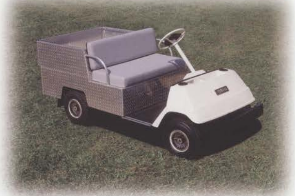
The G1: Yamahauler with G1 (2 Stroke) engine and a diamond plate carrier for large payloads 34" x 43" x 12".
