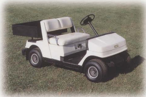
The Black Box: Basic Yamahauler with G1 (2 Stroke) or G2 (4 Stroke) engine and carry box 24" x 39" x 9".
