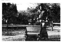
30-12 CORE AERATOR. The self-propelled 30-12 can core up to 13,900 sq. ft./hour; maneuvers easily; and can turn in a 15" radius while aerating.
