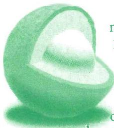
Each Poly-S™ particle is manufactured using a computer-controlled, two-tier coating process that allows nutrients to be released steadily and safely by controlled diffusion through the polymer coating. Thus the rate of release can be regulated over a pre-programmed period of time over a wide variety of weather conditions — providing higher nitrogen analysis than SCU products with less sensitivity to temperature than fertilizers coated with polymer only.
