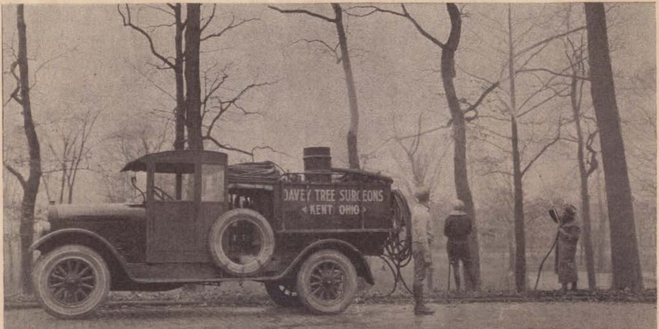
Large tank truck in use applying dormant spray before trees are in leaf. This equipment makes quick work of spraying trees on golf courses, public parks and large estates
