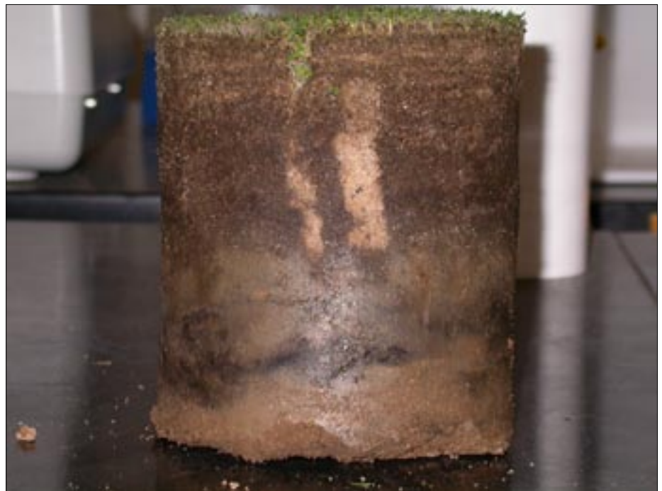
Lack of internal drainage and high levels of organic matter often spell trouble for golf course putting greens for a variety of reasons.
