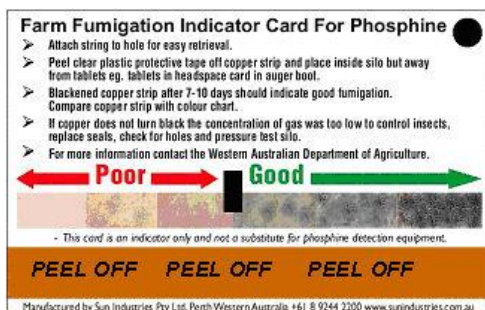
Figure 4. Rear side of the phosphine indicator card with transparent adhesive tape printed with "PEEL OFF" removed from copper strip.
