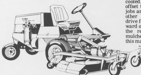
The Groundsmaster 72<sup>®</sup> has power to spare from its water cooled, 4 cylinder engine. The 72" floating cutting deck is offset to handle the bulk of the trimming jobs around trees, along fences, walls and other obstacles. One pedal hydrostatic drive for responsive speed selection in forward or reverse. Optional accessories like the rear discharge cutter deck, leaf mulcher, rotary broom and ROPS make this machine a versatile workhorse.
