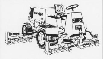
You need a stable machine when you're tackling tough terrain. On bumpy ground. On steep hillsides. Around obstacles. Through dense, wet grass. You need the 5 or 7 bladed Reelmaster® 350-D. Its mid-mounted engine and wide stance create a low center of gravity. And its even weight distribution and six oversized 4-ply tires
