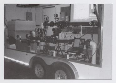
The CIT Pump Demonstration Trailer graphically depicted the advantages and savings of utilizing a VFD pump drive.
