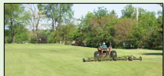
Figure 4. Old technologies such as gang mowers can be highly effective in fuel conservation
