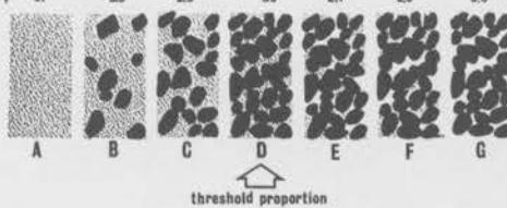
Figure 2. Pictorial diagram illustrating the effect of increasing proportions of coarse-textured amendment on soil water retention, aeration, and compaction resistance.
