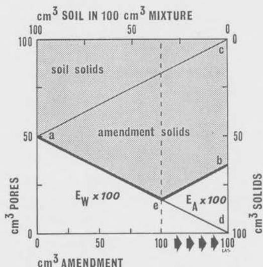
Figure 4. Graphical form of model used to predict soil-mixture physical properties.  $E_W$  equals water retention porosity (in drained golfgreen);  $E_A$  equals aeration porosity;  $a$  equals soil porosity, and  $b$  equals amendment porosity. The dashed line ( $e$ ) is the threshold proportion. The amount of soil in the mix decreases from left to right (proportion of amendment increases). Total porosity equals  $E_W$  plus  $E_A$ .
