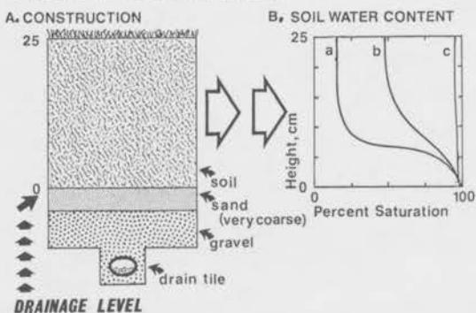
Figure 1. Water distribution pattern (B) for three different "soils" in a typical drained golf green. Soil a equals very coarse-textured sand; c equals silty clay loam; and b equals a mixture of a and c.
