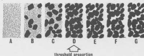
Figure 2. Effect of amendment on soil porosity. The sand is a very coarse-textured river sand. The soil is a silty clay loam. The total bulk volume on the mixture was kept constant.
