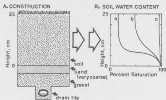
Figure 1. Water distribution pattern (B) for three different soils in a typical drained golf green (A). Soil a = coarse-textured sand; b = a mixture of a and c; c = silty clay loam. All three soils are saturated at the drainage level (perched water table), and the water content decreases with height above this level.
