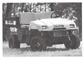
Dual Shocks — MacPherson Struts — Seats 3 Across 4-Wheel Hydraulic Brakes — 1000 lb. Tow Capacity.
