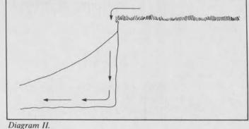
Bunkers constructed in this manner will look better and the sand will definitely stay in place better. This will reduce sand/soil contamination and alleviate the seemingly endless job of replacing washed-out sand after every heavy rainfall.
