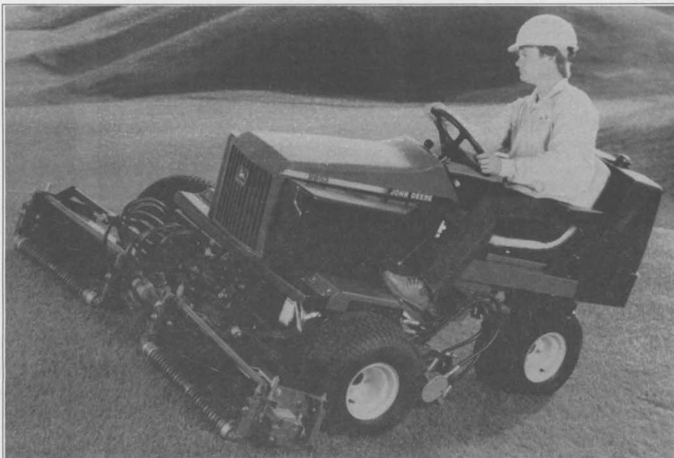
The 2653 features the unique combination of hydraulic reel drive and John Deere 26-inch cutting units.
