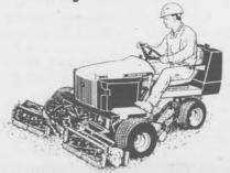
The 2653 features the unique combination of hydraulic reel drive and John Deere 26-inch cutting units.
