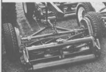
**INDIVIDUAL FRAMING:** Spartan units are individually framed and chain suspended to permit maximum freedom for smoother cutting over undulating turf. Single hand adjustment knob adjusts bedknife against reel.
