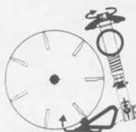
SINGLE KNOB, BEDKNIFE-TO-REEL ADJUSTMENT
