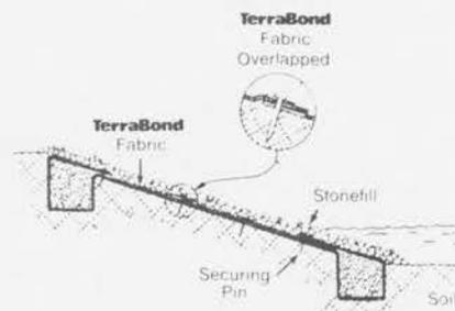
TerraBond is utilized beneath cut slope stone protection (rip-rap) as shown above. The fabric provides long-term confinement of cut slope or fill material.
