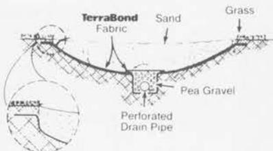
Line the entire golf sand trap with TerraBond, including 6" under the surrounding sod. The sod's roots will knit the fabric to the soil beneath. Clay and rocks will be totally restricted from moving up into the sand.
