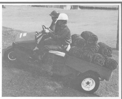
HEAVY DUTY INDUSTRIAL-QUALITY HYDROSTATIC DRIVE gives infinite speed control, instant forward/reverse, high torque to rear wheels for drawbar pull that surpasses competition. It's a closed, self-lubricating drive system as in our Sand Pro and Groundsmaster 72. No gears to change, no clutch to slip.
