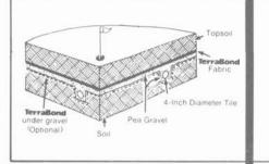
Use TerraBond as a replacement for the usual 2" coarse sand layer between the greens mix and the gravel drainfield. The fabric will eliminate downward migration of the mix into the gravel and the subsequent reduction of water flow from the green.
