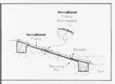
TerraBond is utilized beneath cut slope stone protection (rip-rap) as shown above. The fabric provides long-term confinement of cut slope or fill material.
