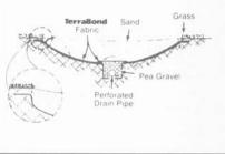
Line the entire golf sand trap with TerraBond, including 6" under the surrounding sod. The sod's roots will knit the fabric to the soil beneath. Clay and rocks will be totally restricted from moving up into the sand.
