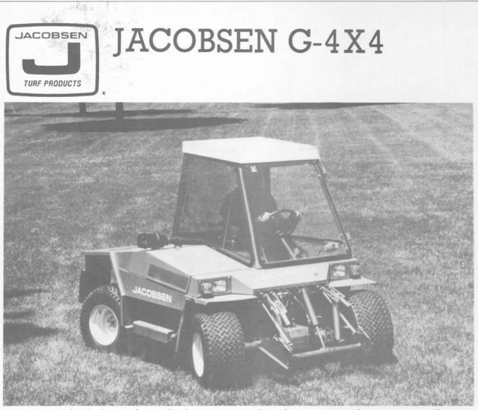
Four-wheel drive, four-wheel steering and a low center of gravity are key features of the Jacobsen G-4X4, a 24 hp diesel-powered machine designed to serve as a mobile power source for rotary and flail mowers, rotary broom and snowthrower, seed and fertilizer spreader and blower. It also has a synchronized eight forward and four reverse speed transmission, four-wheel hydraulic brakes and an all weather cab plus front and rear lights.
