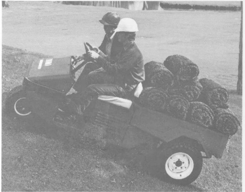
HEAVY DUTY INDUSTRIAL-QUALITY HYDROSTATIC DRIVE gives infinite speed control, instant forward/reverse, high torque to rear wheels for drawbar pull that surpasses competition. It's a closed, self-lubricating drive system as in our Sand Pro and Groundsmaster 72. No gears to change, no clutch to slip.
