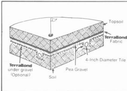
Use TerraBond as a replacement for the usual 2" coarse sand layer between the greens mix and the gravel drainfield. The fabric will eliminate downward migration of the mix into the gravel and the subsequent reduction of water flow from the green.
