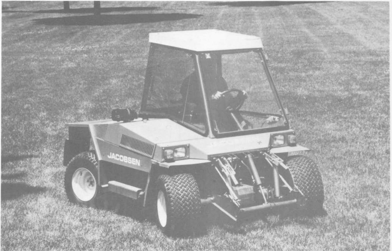
Four-wheel drive, four-wheel steering and a low center of gravity are key features of the Jacobsen G-4X4, a 24 hp diesel-powered machine designed to serve as a mobile power source for rotary and flail mowers, rotary broom and snowthrower, seed and fertilizer spreader and blower. It also has a synchronized eight forward and four reverse speed transmission, four-wheel hydraulic brakes and an all weather cab plus front and rear lights.
