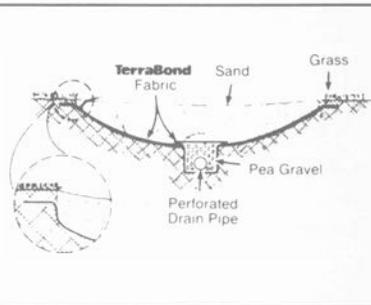
Line the entire golf sand trap with TerraBond, including 6" under the surrounding sod. The sod's roots will knit the fabric to the soil beneath. Clay and rocks will be totally restricted from moving up into the sand.
