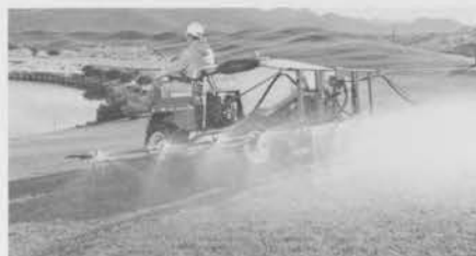
The 1800 Utility Vehicle brings the benefits of hydrostatic drive to spraying and spreading jobs.
