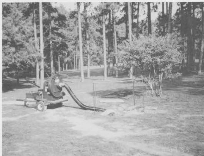
Subair system is used to pull moisture from top 3-4 inches of the soil to help firm up and increase green speed
