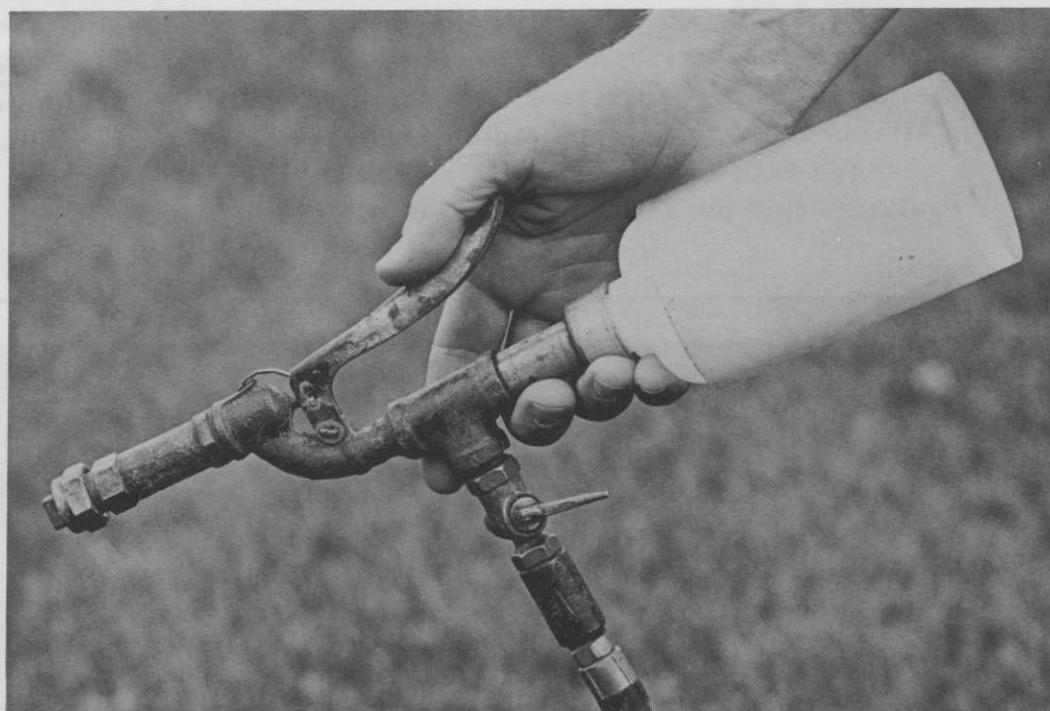
Figure 2. Close-up of spray unit and container (plastic Nalgene bottle with sleeve).
