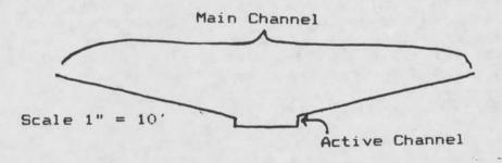
Figure 1: Stream channel as designed for Alvamar.
