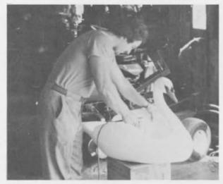
Our Mechanic, Art Schremeck, drilled a total of eight holes in the bottom of the body, 13/32" large. Art tells me that the holes should be reamed with a hot poker to smooth the walls so the rough surface can't trap debris, eventually plugging the holes.
