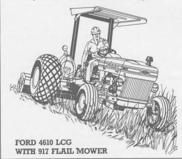
Ford LCG tractors are especially designed for mowing on slopes. With their wide-set axles and low center-of-gravity, they really hug the ground.
