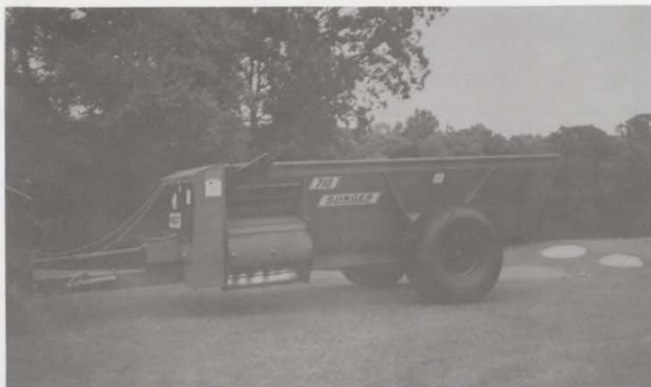
A view of the Knight 710 Slinger manure spreader's flair-type discharge device, which slings clippings up to 45 feet into the roughs, offering a tidy solution to clipping disposal.
