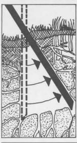
Fractures and lifts compacted soil
