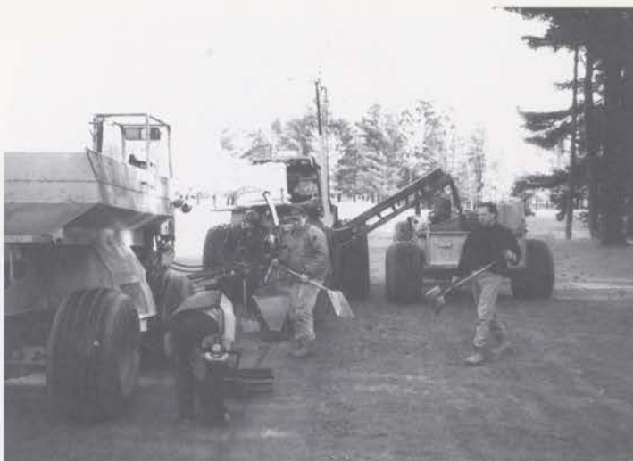
Specialized equipment installing 1.5-inch-diameter slit drains in a one-pass operation.
