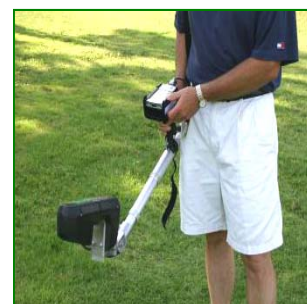
"GreenSeeker" handheld sensor collects data and records it to a spreadsheet in a PDA as the operator travels across the turfgrass. Photo by Greg Bell
