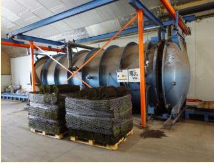
Direct Gazon vacuum machine for chilling grass for shipment.
